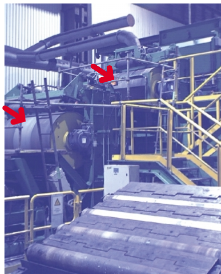
Figure 3: S-Pair of rollers (arrows), one roller in two is encased. An S-pair of rollers is used for pulling the tape through the facility (cf. Figure 4)
