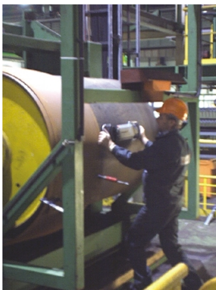
Figure 2: Measuring a roller with PARALIGN®
